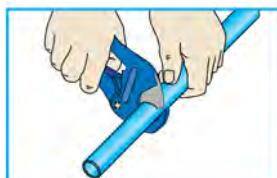
DO NOT use a hacksaw. To avoid damage to the O-ring remove burrs and sharp edges.
