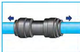
To disconnect, ensure the system is depressurized. Push the collet towards the fitting and remove the pipe. The fitting can be reused.
